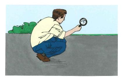
Your driveway may look smoother in some areas than in others because of the makeup of asphalt. Asphalt has various sizes of stone, sand, liquid asphalt, and other ingredients which cause a varied texture of the surface. Also, driveway areas that have been raked and spread with hand tools may appear different in texture from those spread by machine.
